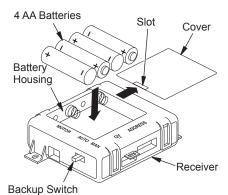
Figure 33 - Installing Batteries in Receiver
